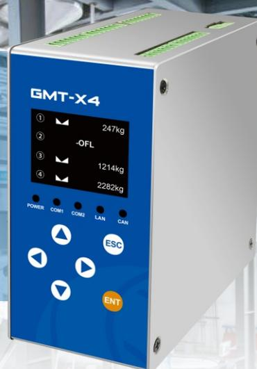
GMT-X4 is a DIN rail mounted weighing transmitter with four-channel. It has the characteristics of compact design, stable performance, and easy operation, which can be used for various weighing applications, such as weight checking, loss-in-weight, liquid filling, batching, vessel and silo weighing, etc.
